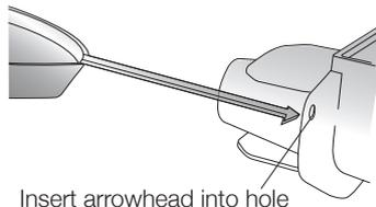
Insert arrowhead into hole on side of Flo-Tone, from behind.
