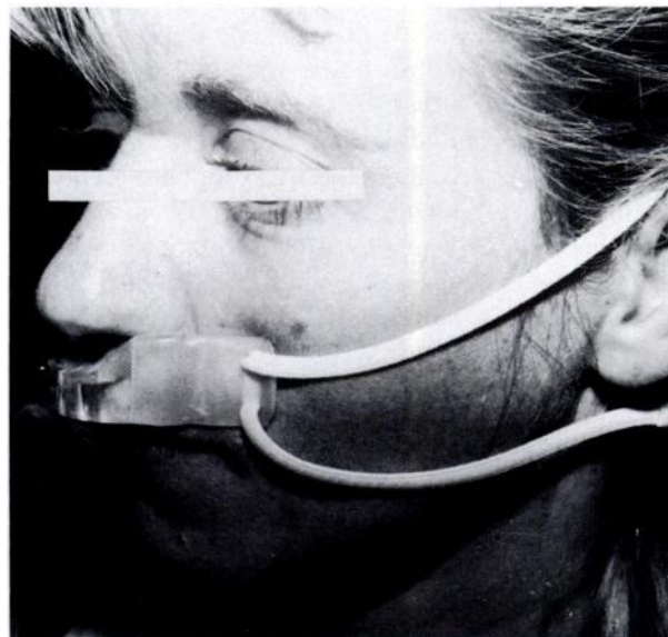
FIGURE 4. Oxygen flow at the outlet made visible by cigarette smoke (flow, 2 L/min). Nearly all the smoke is inhaled by mouth breathing.
